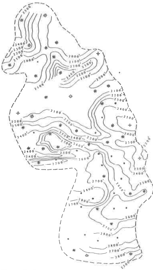
Figure 7. Structure contour map of upper surface of subsurface Mississippian Monteagle Limestone.
