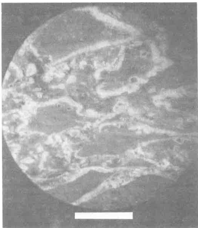
Figure 3. Matrix of sample SK-88-9, Catoctin breccia 1.5 km north of The Plains, Virginia on Highway 626 ("Low-Ti metabasalt breccia" of Espenshade, 1986). Clasts (not seen) range from fist size to <1 cm and are composed of tremolite > epidote > albite(?) > sphene. These have no rimming effect. Matrix grains (those shown) range from almost 1 cm to <1 mm and are composed of epidote > chlorite > albite(?). These have rims enriched in sphene and epidote. The smallest grains are entirely of the rim composition. The mesostasis consists of variable amounts of chlorite + calcite + quartz + tremolite. Scale bar represents 5 mm.
