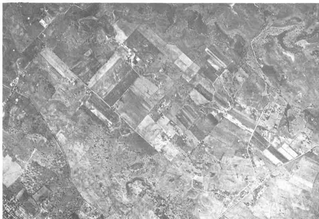
Figure 3: Low-altitude aerial photograph showing stratigraphic strike (locally N 29°E) by alignment of fields, roads, and valleys. North is toward right of photo; left edge of photo covers 3.0 km.
