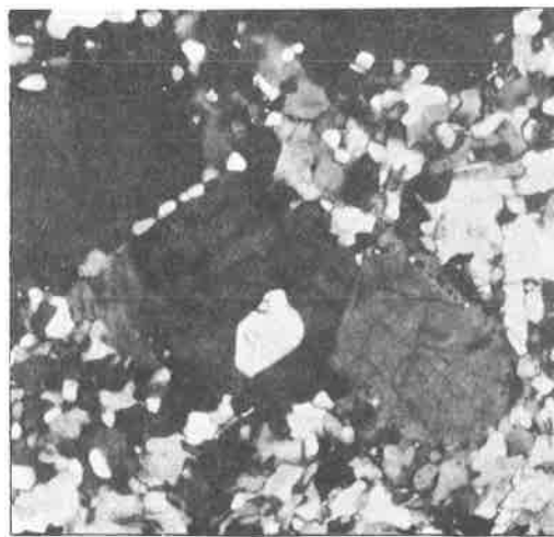
Figure 3. Photomicrograph showing subhedral quartz inclusion in plagioclase phenocryst; field of view approx. 3 mm.
