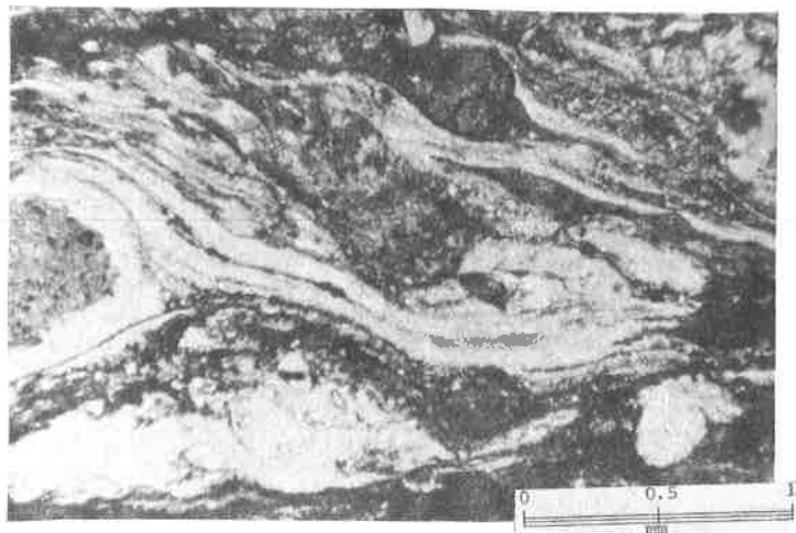
Figure 6. Photomicrograph of mylonite developed in adamellite. Augen of epidote (dark) and sericitized feldspar (gray) are surrounded by ribboned quartz.
