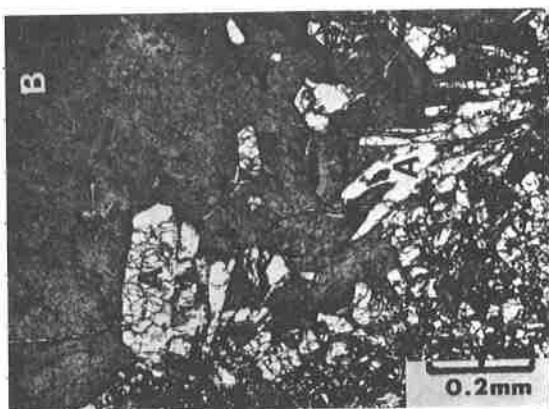
Figure 3. Photomicrograph of gypsum crystals (A) growing centripitally from the margin of a dolomite lined void that later completely filled in with ferroan calcite (B). Daus section (D-2-2), alizarin red stain, uncrossed nicols.
