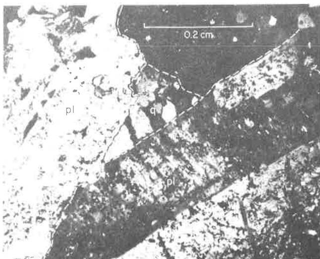
Figure 3. a. (top) Photomicrograph of zoned, subhedral plagioclase (saussuritized) in medium-grained biotite quartz biorite (unit b) of the Port Deposit Gneiss. b. (bottom) Photomicrograph of wedge-shaped interstitial quartz (q) between subhedral plagioclase crystals in unit b of the Port Deposit Gneiss.
